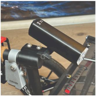
**A7.** Push the slotted bracket of the light into the slots of the holder and make sure they are aligned. Seen in the traveling direction of the Walker, enter the included wingnut from the left and tighten it.
